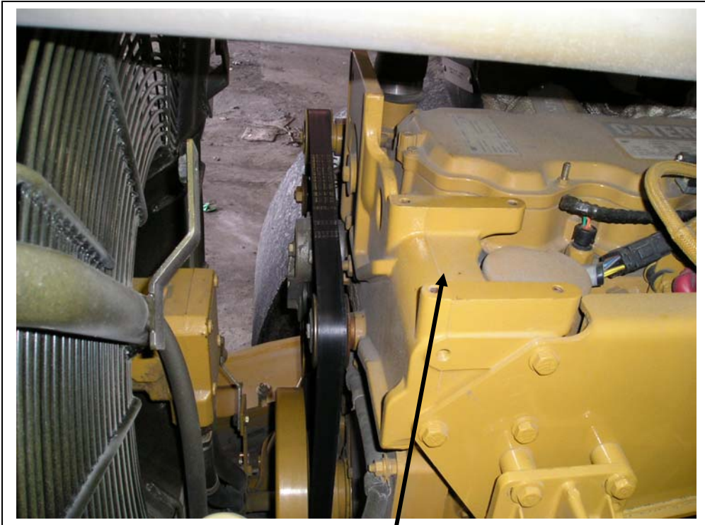
Direct mount compressor location. Uses factory AC belt and additional backside idler pulleys.
