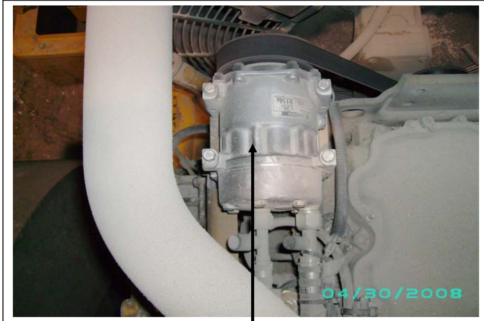
Compressor shown in place with belt and hoses connected.
