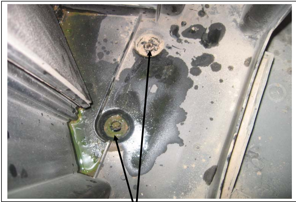
Split the unit and remove the drain plugs.
