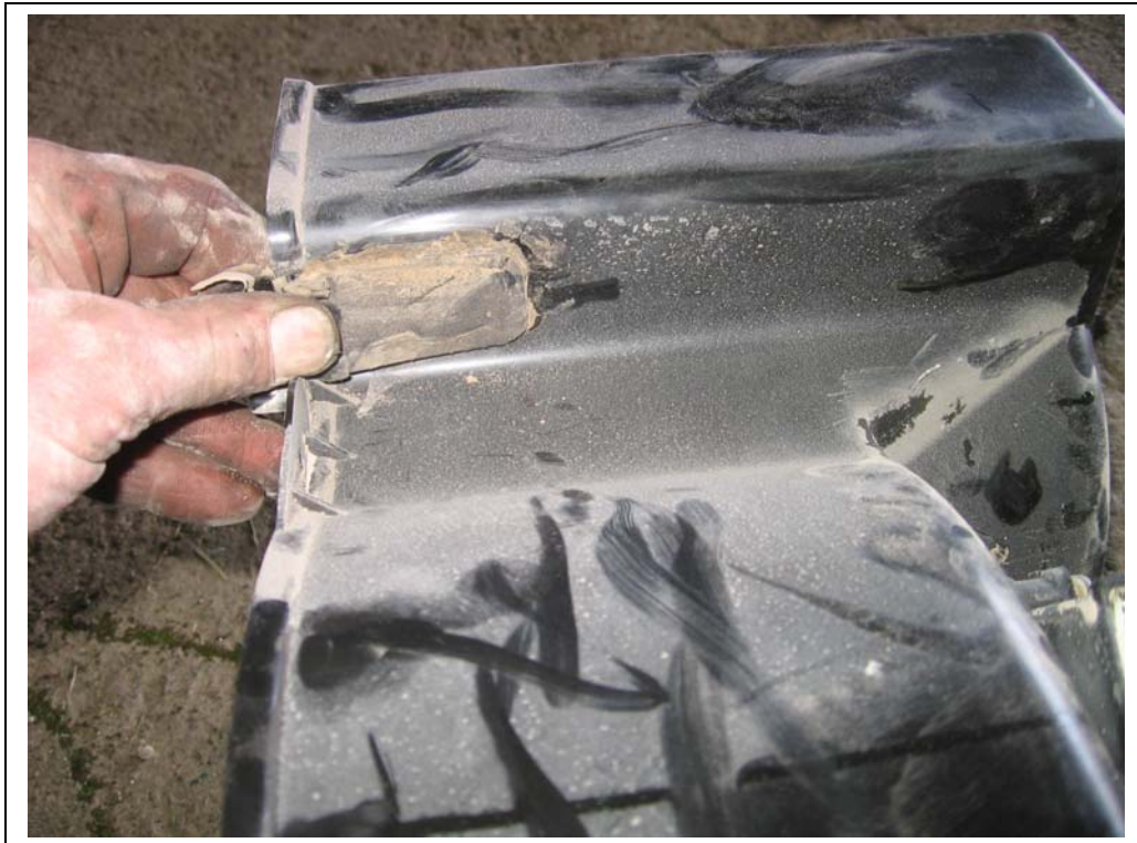
Remove rubber grommets from the lid as shown. This is where the evaporator fittings will come out. Install the evap coil into the box then fit the lid over it. This coil fits tight and likely some plastic will need to be cut around the fitting area.
