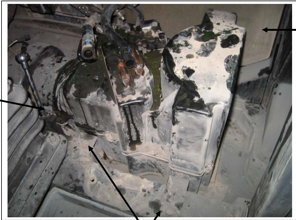
Remove heater assembly from unit. (3 bolts)
