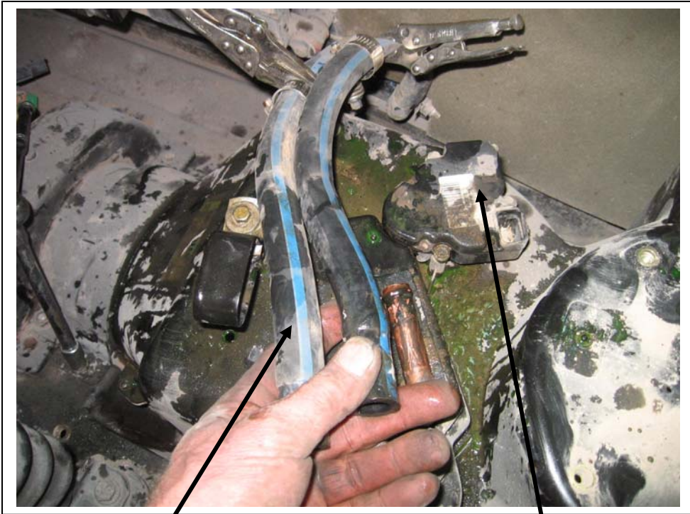
Pinch the heater lines and remove from the unit as shown.
